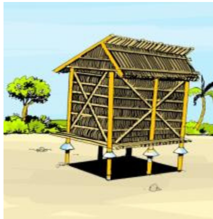
Figure 2.13: An improved drying crib
