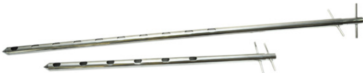
Figure 2.4: Multi-compartment sampling spears (160cm or 102cm) to sample bulk grain from various depths
